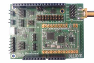
A remote management solution for public lighting. The RDS - LIGHT solution is a FM-based control system that optimises public lighting and allows local autorities and electrical operators to see any malfunctions in real time.
