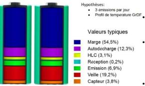
The energy dimensioning of a sensor: a compromise between functionality, cost and lifetime.
